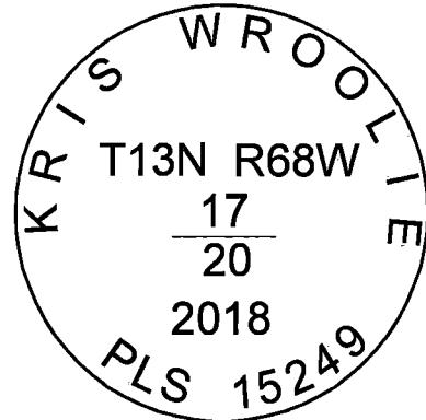
**RESET:** Set aluminum capped monument stamped LS 15249 at lost location between the NE and NW corners of section 20
